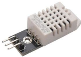
Fig. 2 : DHT22 Temperature & Humidity Sensor DHT22 (n.d.).
